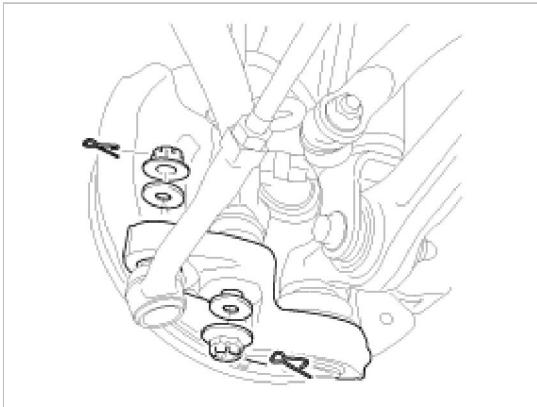
2. Disconnect the tension arm (A) with the front knuckle using a SST (09568-2J100).
