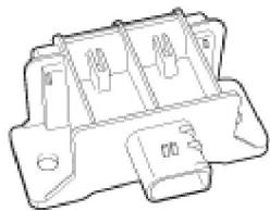
Initiators are used to radiate magnetic energy to the wheel sensors. The wheel initiators are used to communicate with the TPM wheel sensors. The wheel initiators receive a low energy control signal from the receiver. This signal is amplified and radiated as magnetic energy to initiate RF response from a wheel sensor.
